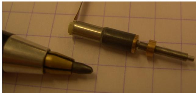
Figure 8: Example of a micro motor used for calibration
