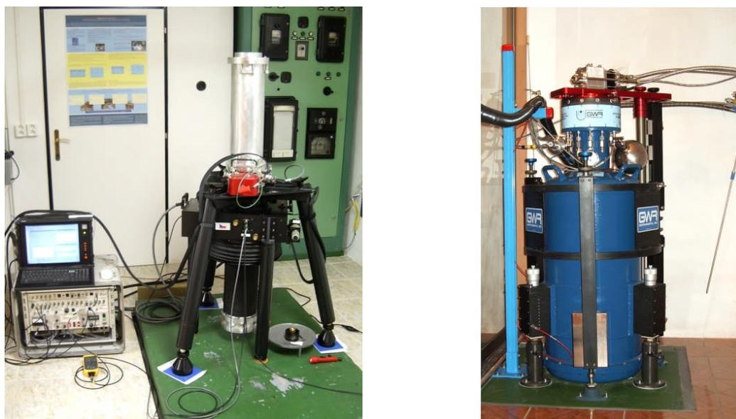
Fig. 1. The absolute gravimeter FG5#215 and the superconducting gravimeter OSG-050 at the Pecný station
