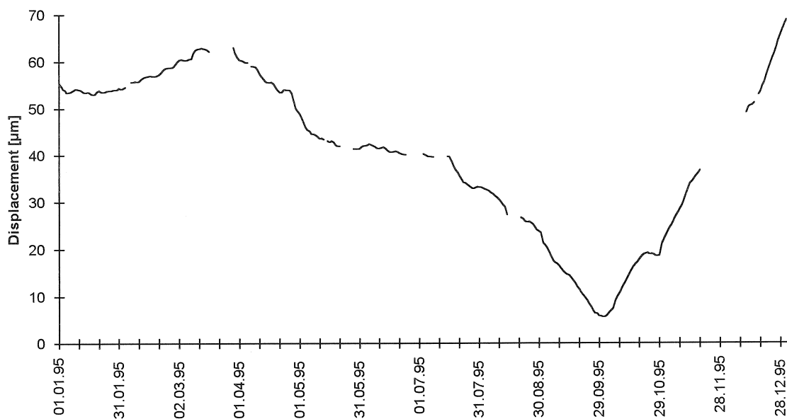
Fig. 6. Deformation measured by the quartz tube extensometer in Pécs in 1995
