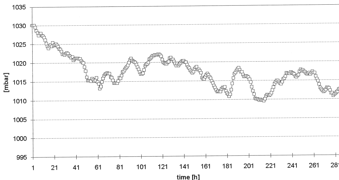
Fig. 2. Air pressure recorded by the microbarograph in the time interval 20.05.92. - 01.06.92.
