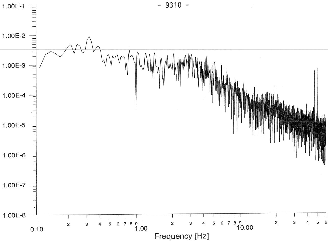
*fig. 4: Membach, exemple of spectrum (vertical component) taken when the refrigerating device is on.
