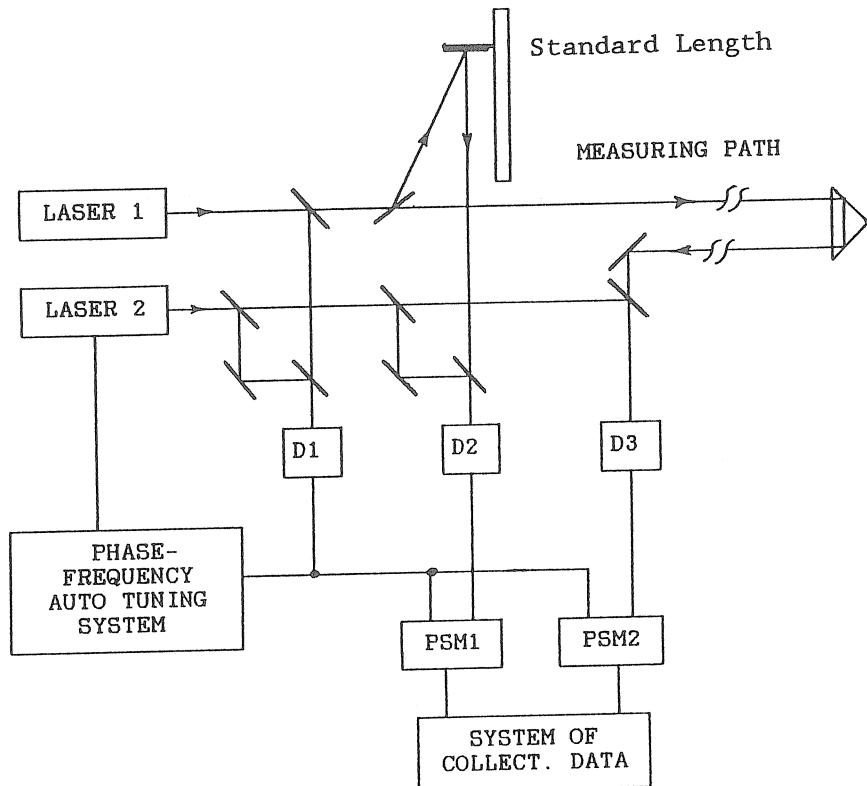
Fig. 1. Schematic diagram of the laser extensometer, with one measuring leg.
