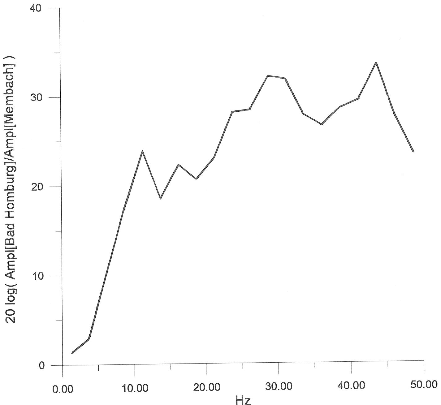
Fig. 10 : comparison (in db) of the noise in Bad Homburg (March 94) with the noise in Membach (June 94) which is the reference. The refrigerating device is off. Each point is an average of the amplitude on a 2.5 Hz interval.
