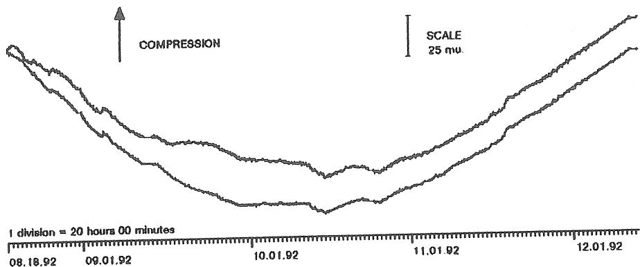
**Fig. 4.** Time change of relative deformation that was registered along measuring legs 1 and 2 of the laser deformograph from 18.08.92 to 11.12.92.
