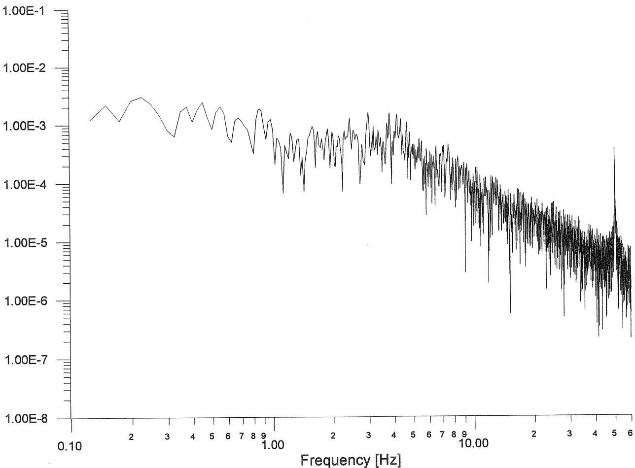
*Fig.5 : Membach, spectrum of the noise (vertical component), when the refrigerating device
