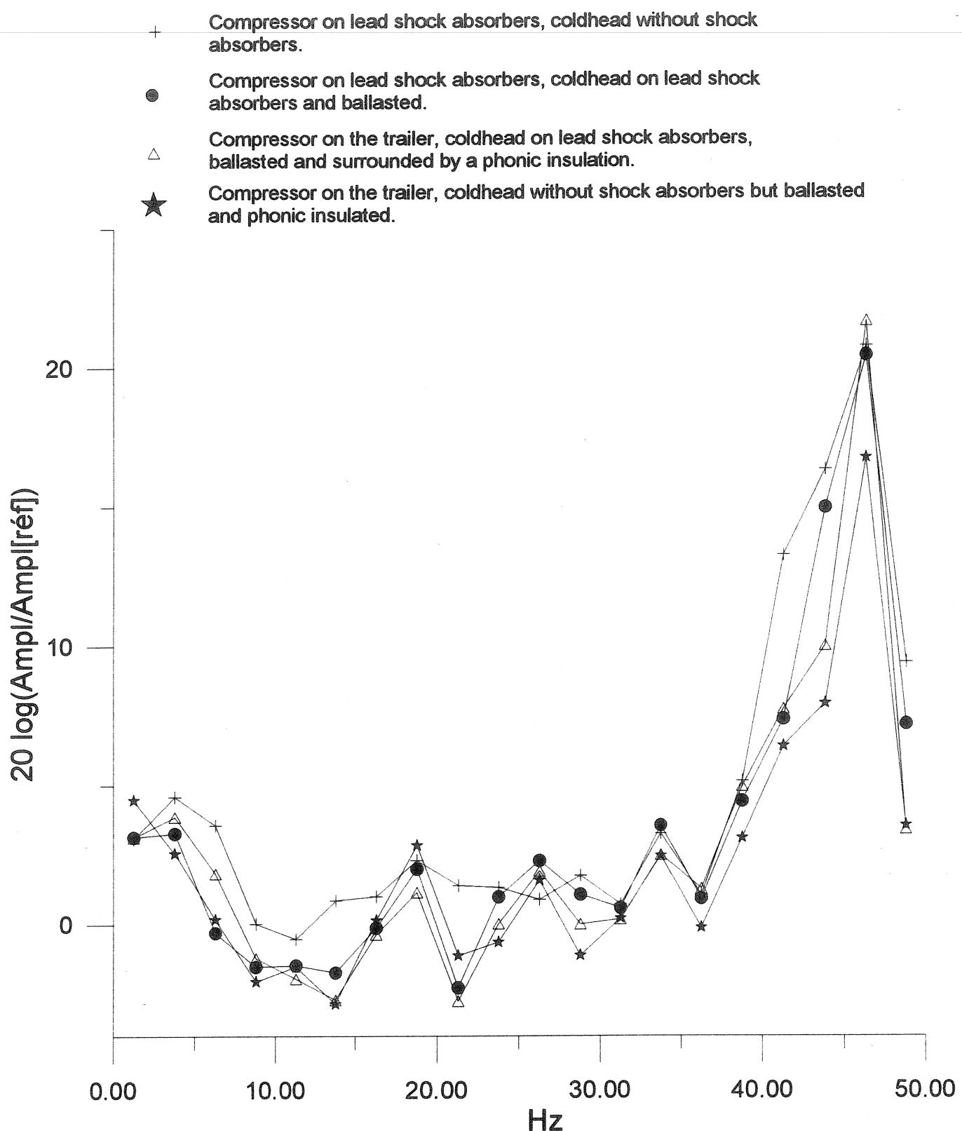
Fig. 8 : Membach : horizontal component (east-west) : compaison (in dB) of a reference spectrum with the spectra calculated for different shock absorbers placed beneath both the compressor and the coldhead. The compressor is at 100 m from the seismometers and the coldhead at 15 m.
