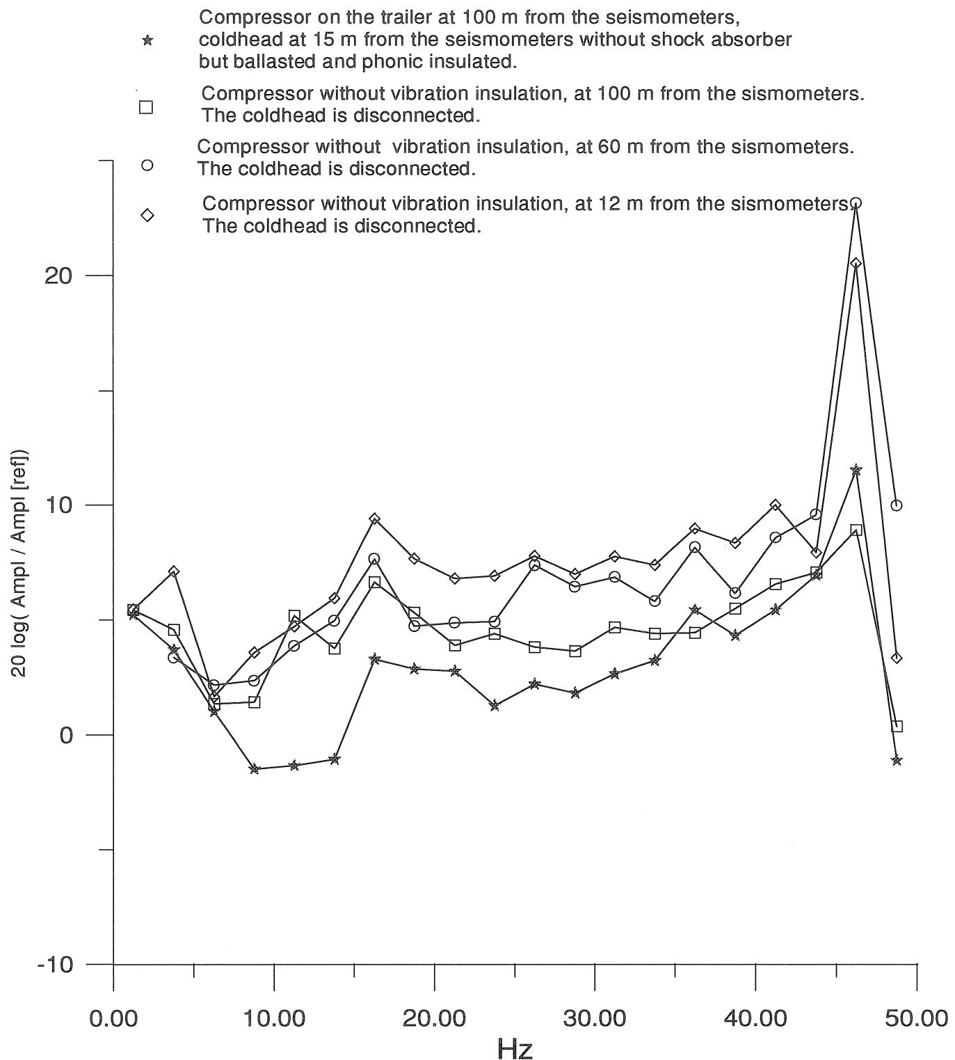
Fig.3 : Membach : vertical component : comparison (in dB) of a reference spectrum with the spectra calculated for different distances of the compressor to the sismometer. There is no shock absorber below the compressor. The reference spectrum is calculated when no compressor is present. The comparison when the compressor is on the trailer is also shown as it has the best noise level.
