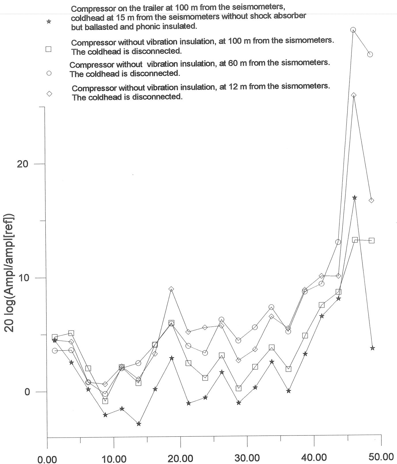
Fig.9 : Membach : horizontal component (east-west) : comparison (in dB) of a reference spectrum with the spectra calculated for different distances of the compressor to the sismometers. There is no shock absorber below the compressor. The reference spectrum is calculated when no compressor is present. The comparison when the compressor is on the trailer is also shown as it has the best noise level. Each point is an average of the amplitude on a 2.5 Hz interval.
