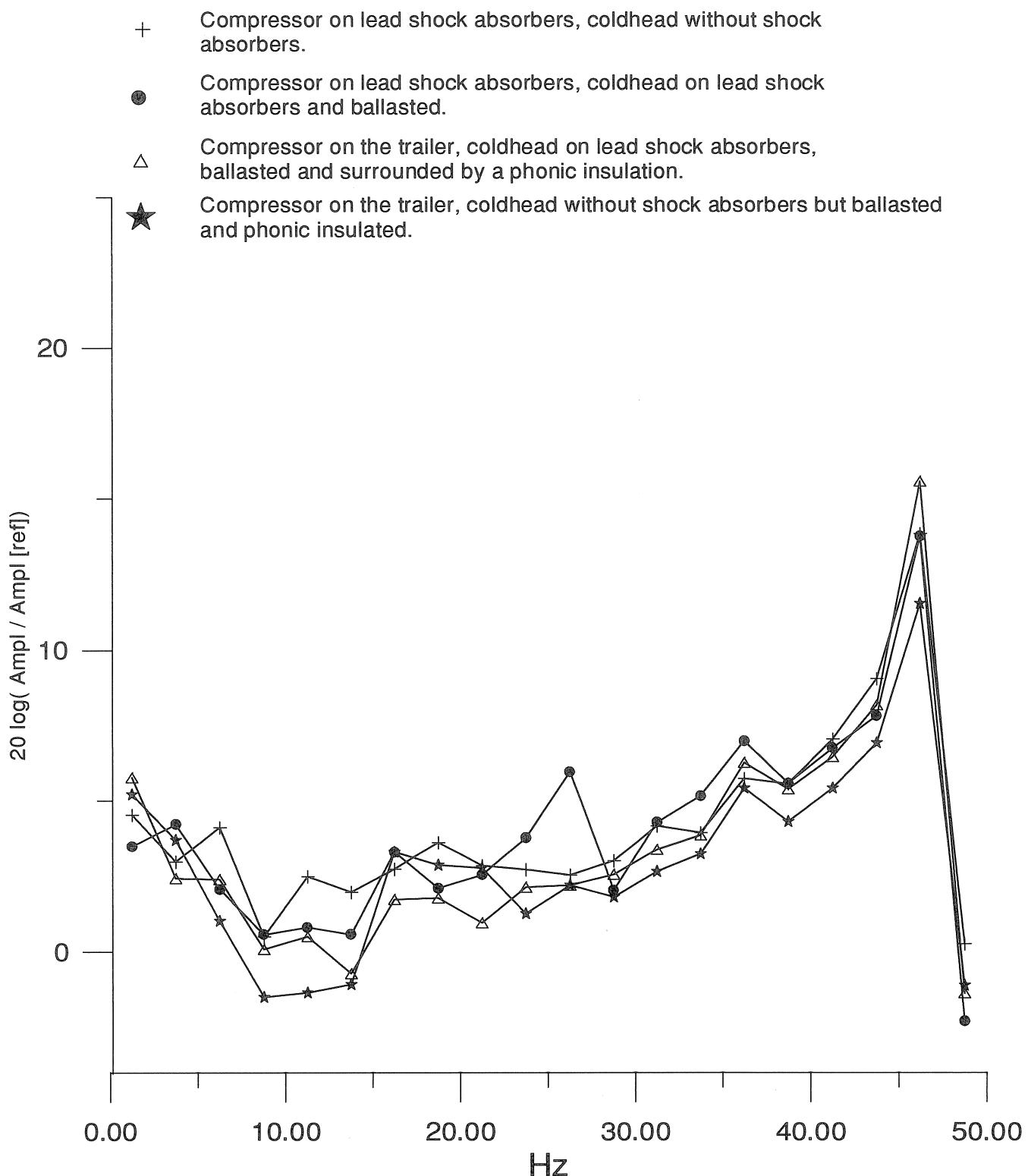
Fig.2 : Membach : vertical component : comparison (in dB) of a reference spectrum with the spectra calculated for different shock absorbers placed beneath both the compressor and the coldhead. The compressor is at 100 m from the seismometers and the coldhead at 15 m. The reference spectrum is calculated when no compressor is present. Each point is an average of the amplitude on a 2.5 Hz interval.
