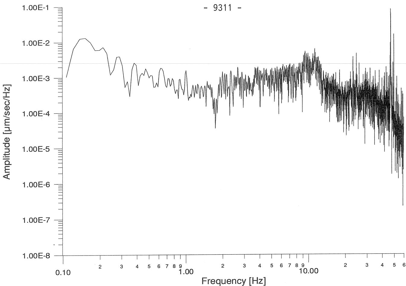
*fig. 6: Bad Homburg, spectrum of the noise (vertical component) when the refrigerating device is on. The sismometer is on a pillar at 3 m from the compressor. Note the 47.2 Hz peak.*
