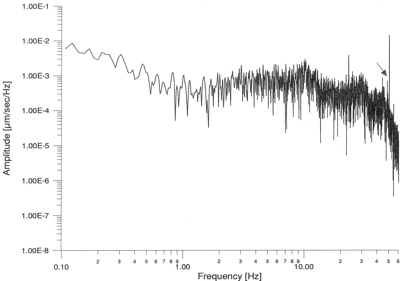
*fig. 7: Bad Homburg, spectrum of the noise (vertical component), when the refrigerating device is off. Note the presence of the 50 Hz peak and the absence of the 47.2 Hz one. The peak near the 50 Hz one, indicated by an arrow, is not on 47.2 Hz.*
