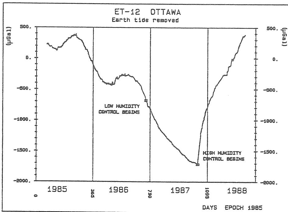
Figure 3. Drift history of ET-12 since 1985, in normal and controlled environments.
