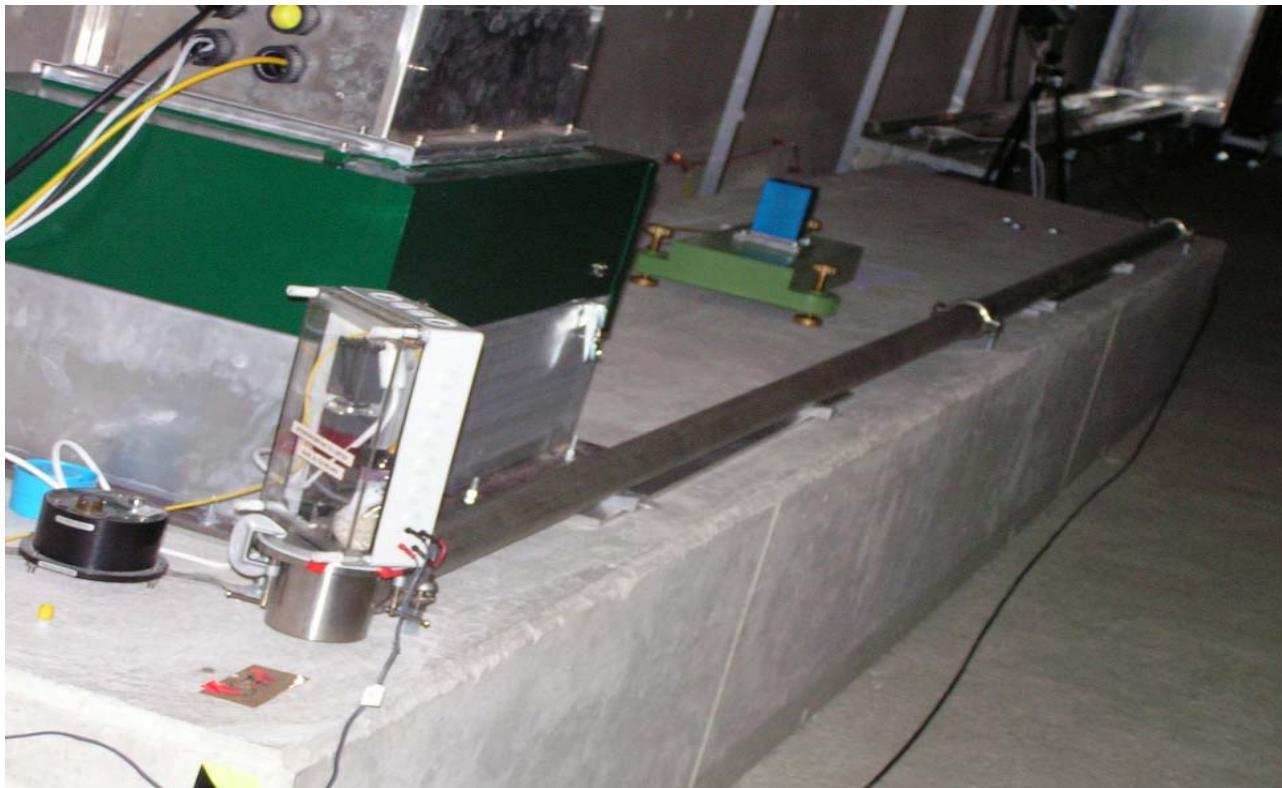
**W\_iWT** tilt meter **one end prototype** recording
