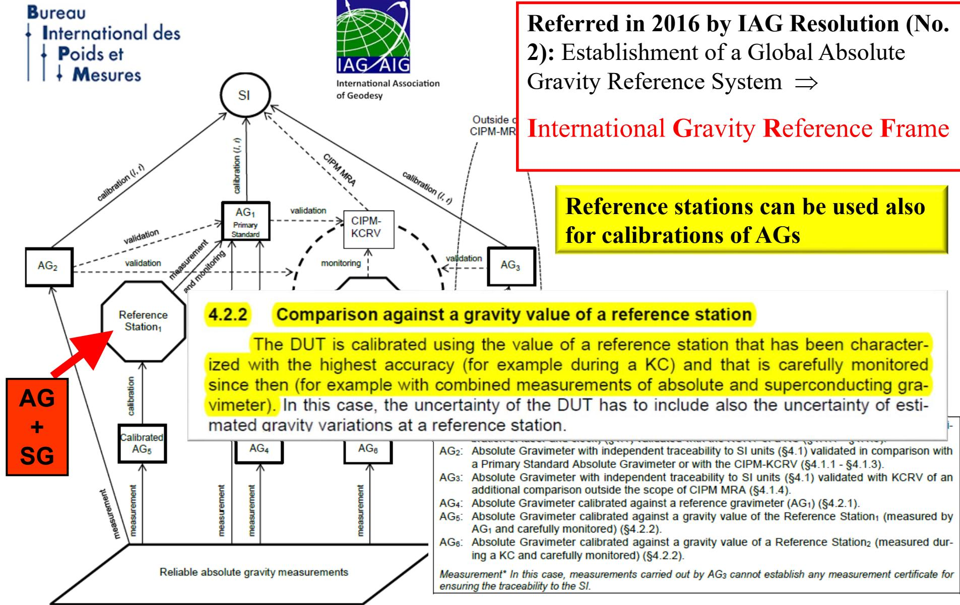
Figure 1: Scheme of the traceability chain in gravimetry, according to §§4.1 – 4.2.
